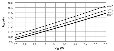
Figure 31-14. Idle Supply Current versus  $V_{CC}$  $f_{SYS} = 32MHz$  Internal Oscillator
