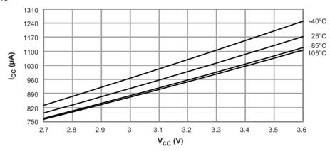
Figure 31-6. Active Supply Current versus  $V_{CC}$  $f_{SYS} = 32MHz$  Internal Oscillator Prescaled to 8MHz
