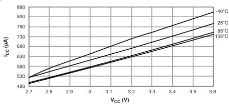
Figure 31-4. Active Supply Current versus  $V_{CC}$  $f_{SYS} = 32.768$ kHz Internal Oscillator
