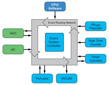
The event routing network consists of four software-configurable multiplexers that control how events are routed and used. These are called event channels, and allow for up to four parallel event routing configurations. The maximum routing latency is two peripheral clock cycles. The event system works in both active mode and idle sleep mode.
