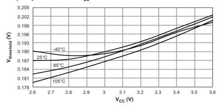
Figure 31-27. Reset Input Threshold Voltage versus  $V_{CC}$   $V_{IH}$  - Pin Read as "1"
