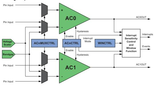
The window function is realized by connecting the external inputs of the two analog comparators in a pair as shown in Figure 25-2.
