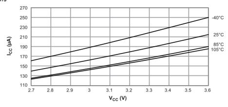
Figure 31-5. Active Supply Current versus  $V_{CC}$  $f_{SYS} = 2MHz$  Internal Oscillator
