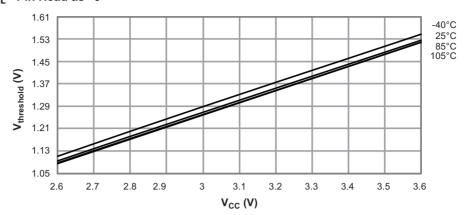
Figure 31-26. I/O Pin Input Hysteresis versus  $V_{CC}$
