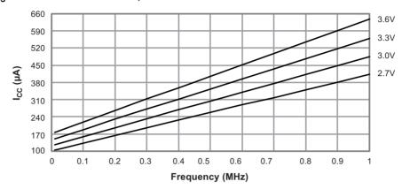
Figure 31-2. Active Supply Current versus Frequency  $f_{SYS} = 1 - 32MHz$  External Clock,  $T = 25^{\circ}C$
