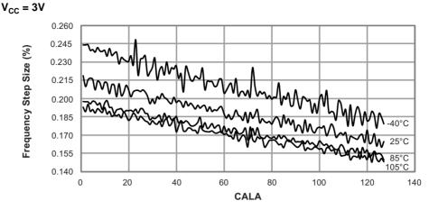
Figure 31-32. Internal 2MHz Oscillator CALB Calibration Step Size  $V_{CC}$  = 3V, CALA = Mid Value
