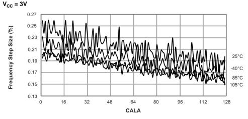
Figure 31-34. Internal 32MHz Oscillator CALB Calibration Step Size  $V_{CC}=3V,\,CALA=Mid\,Value$
