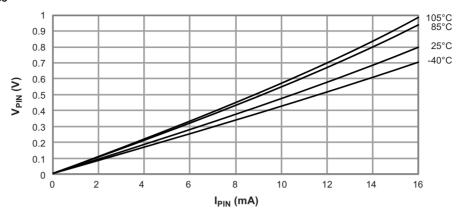
Figure 31-23. I/O Pin Output Voltage versus Sink Current
