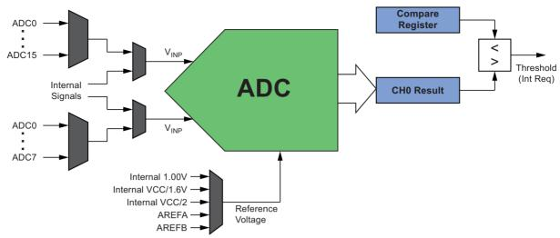
The ADC may be configured for 8- or 12-bit result, reducing the minimum conversion time (propagation delay) from 3.35µs for 12-bit to 2.3µs for 8-bit result.
