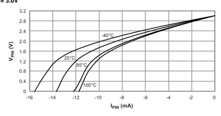
Figure 31-21. I/O Pin Output Voltage versus Source Current  $V_{\text{CC}} = 3.3V$
