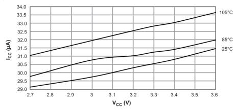
Figure 31-12. Idle Supply Current versus  $V_{CC}$  $f_{SYS} = 2.0 MHz$  Internal Oscillator
