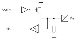
Figure 13-6. I/O Configuration - Wired-AND with Optional Pull-up
