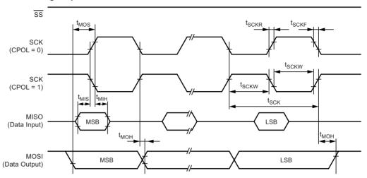
Figure 30-6. SPI Timing Requirements in Slave Mode
