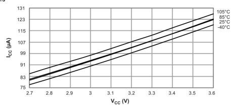
Figure 31-11. Idle Supply Current versus  $V_{CC}$  $f_{SYS} = 32.768 kHz$  Internal Oscillator
