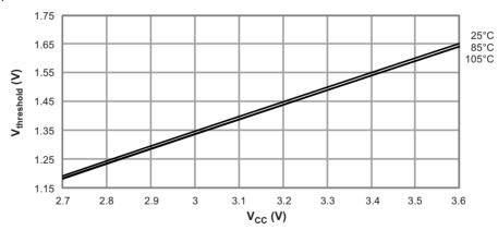
Figure 31-28. Reset Input Threshold Voltage versus  $V_{CC}$   $V_{II}$  - Pin Read as "0"
