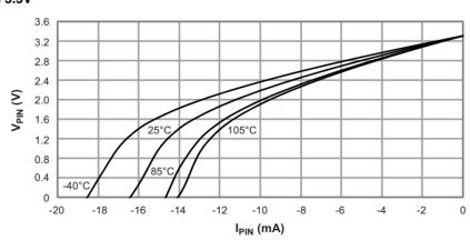
Figure 31-22. I/O Pin Output Voltage versus Sink Current
