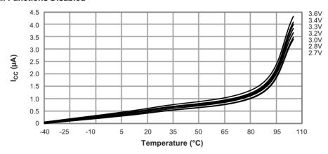
Figure 31-16. Power-down Supply Current versus Temperature
