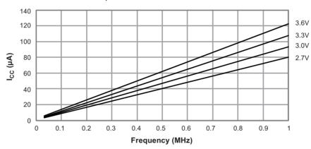
Figure 31-9. Idle Supply Current versus Frequency  $f_{SYS} = 1 - 32MHz$  External Clock, T = 25°C
