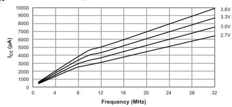
Figure 31-3. Active Supply Current versus  $V_{CC}$   $f_{SYS} = 1 MHz$  External Clock
