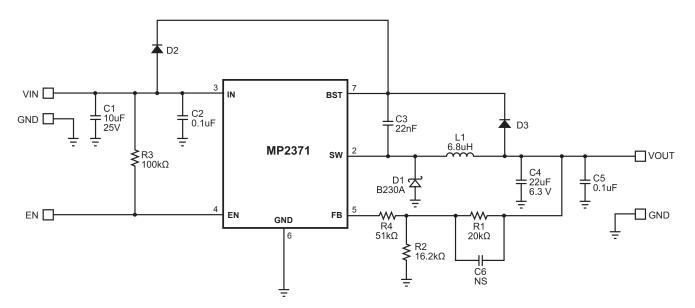
Figure 4—700KHz, 3.3V Output Step-Down Converter
