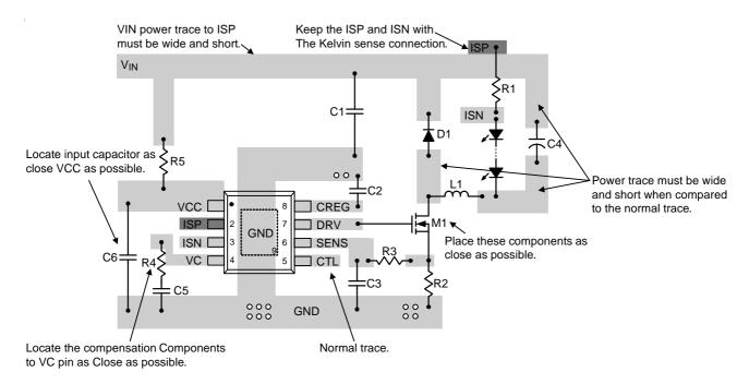
Figure 2. PCB Layout Guide
