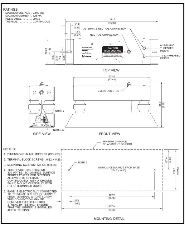
FIGURE 5. PGE-05KV Sensing Resistor.
