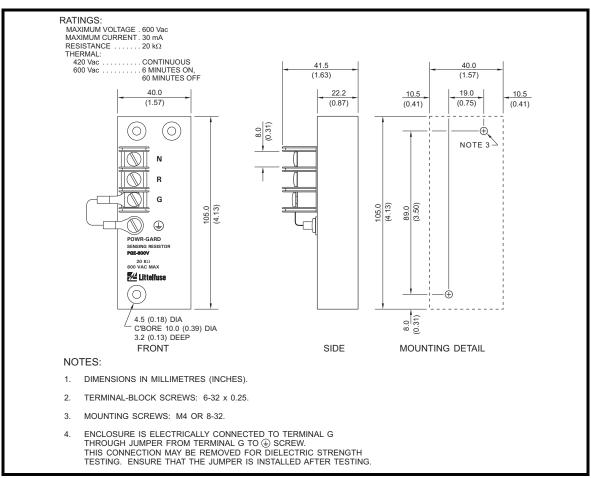
FIGURE 4. PGE-600V Sensing Resistor.
