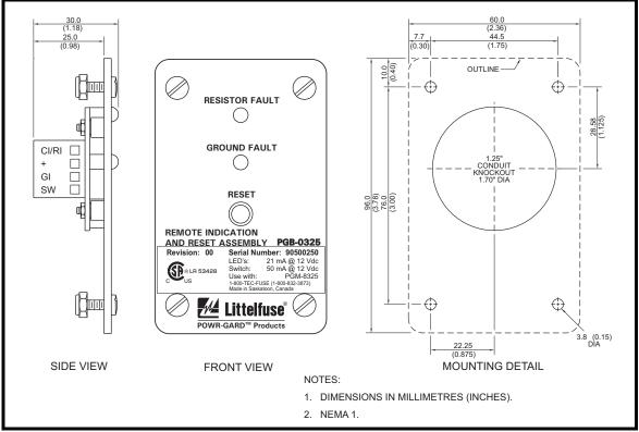
FIGURE 9. PGB-0325 Remote Indication-and Reset Assembly.
