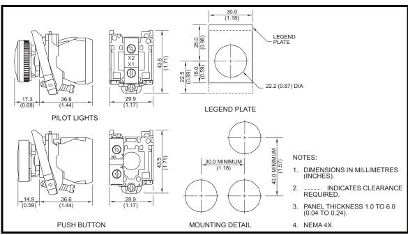
FIGURE 8. PGB-0302 Remote Indication and Reset.
