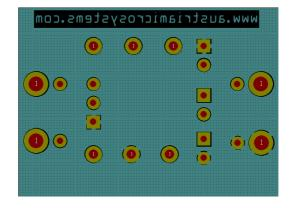
Figure 6: Top + Bottom Layer (adjustable Vout)
