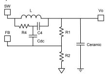
Figure 12—Simplified Circuit of Ceramic Capacitor with DC blocking capacitor
