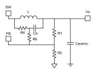
Figure11—Simplified Circuit of Ceramic Capacitor
