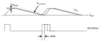
Figure 5—Jitter in Skip Mode
