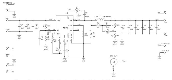
Figure 15 — Typical Application Circuit with Low ESR Ceramic Output Capacitor  $V_{\text{IN}}$ =7-22V,  $V_{\text{OUT}}$ =5V,  $I_{\text{OUT}}$ =6A
