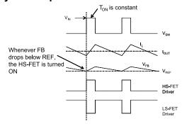
Figure 2—Heavy Load Operation
