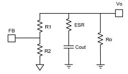
Figure 8—Simplified Circuit in skip Mode
