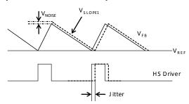
Figure 4—Jitter in PWM Mode
